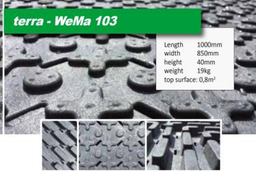
Features: tongue and groove system, simple, self-contained installation. Like the LoMa, provides all the advantages of an extensive drainage.
